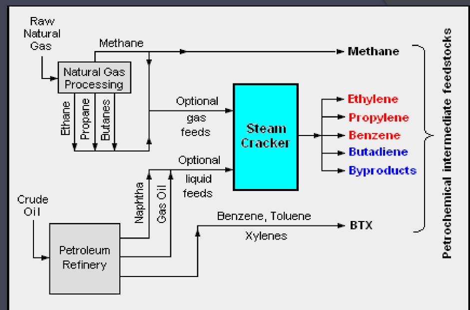
Produced by cracking any of the optional feeds.
